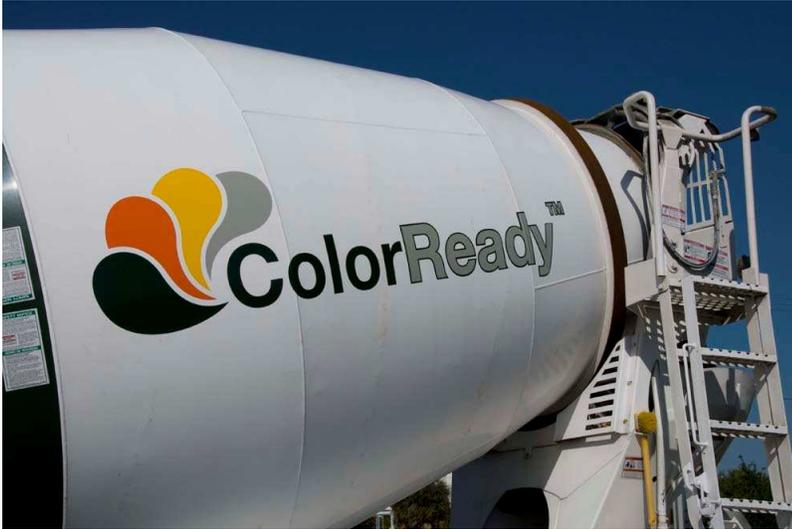
As innovators in ready mixed concrete, block, and other building materials, Preferred Materials has created ColorReady™, a liquid pigment integrally colored concrete.
